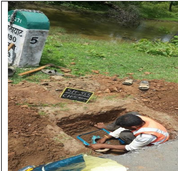
Field Density by Sand Replacement Test in progress
